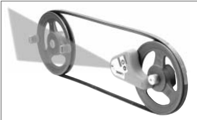
Mounted in a few seconds, the laser line projected on the targets allows you to quickly ascertain and correct misalignment. The TEXROPE® ATX identifies parallel as well as angular misalignment between the pulleys and is suitable for pulley diameters of 60 mm and larger. It is so light it can be mounted on non-magnetic pulleys with the double sided adhesive tape and used on both horizontally and vertically mounted machines.
