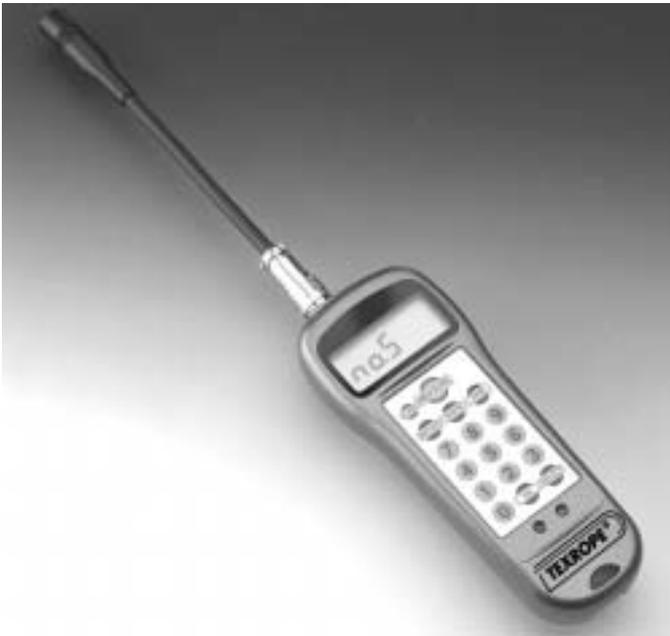
The sonic tension meter measures tension by analysing the sound waves, which the belt produces when strummed. A belt vibrates at a particular frequency based on its static tension, the belt mass and the free span. The tension tester transforms this frequency in a tension value.
